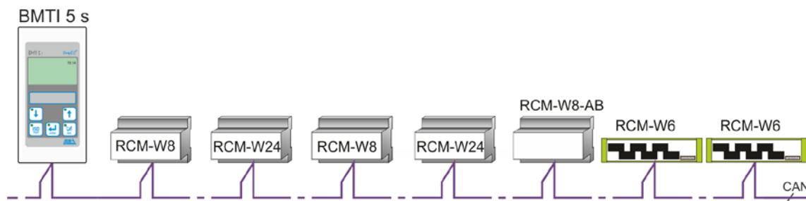
Residual and operating current monitoring with multi-channel power monitoring devices (selection)
